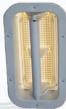
Sidewall vent - Squeeze handle and rotate to open/close
